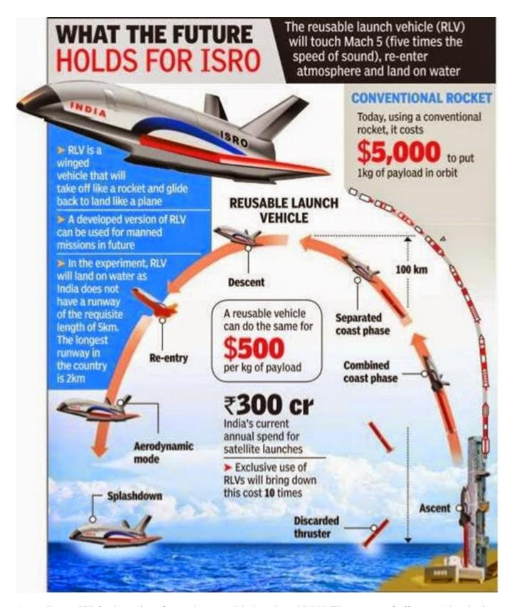
According to ISRO, the series of experiments with the winged RLV-TD are part of efforts at "developing essential technologies for a fully reusable launch vehicle to enable low-cost access to space".
